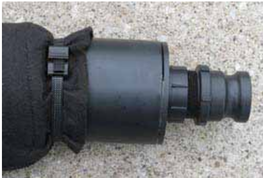
Two-inch Camlock quick connect fitting.
